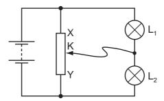
The contact K is halfway between X and Y and the lamps are equally bright.
