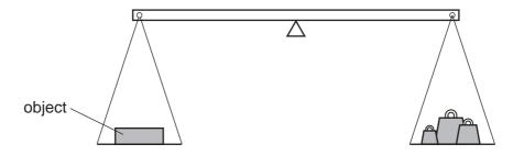
The object is put in the left-hand pan and various standard weights are put in the right-hand pan. These are the results.
